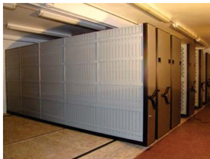
CABINETS ON HIGH DENSITY
